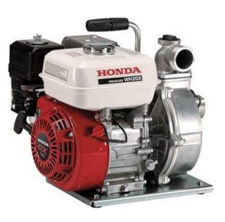
WH20X - This is a high output, high pressure pump with a strong 5.5HP OHV engine, with 50mm (2") ports and a maximum capacity of 500 litres per minute.
