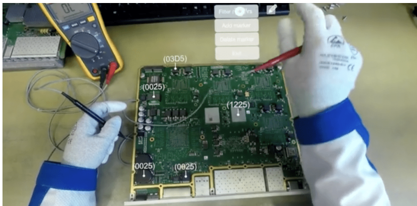
A technician repairs a circuit board using an augmented reality overlay at Ericsson's Tallinn factory. (Source: Ericsson )
