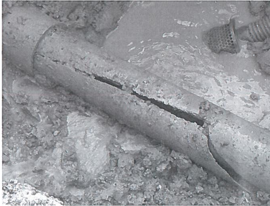
Figure C-3: Longitudinal watermain break with evident Contamination .
