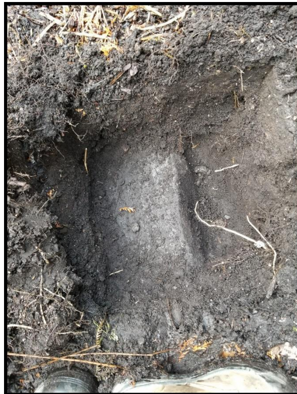
Image 8. Photograph 2557 of the test pit dug in the garden bed on the eastern portion of the study area, showing geotextile over bedrock.
