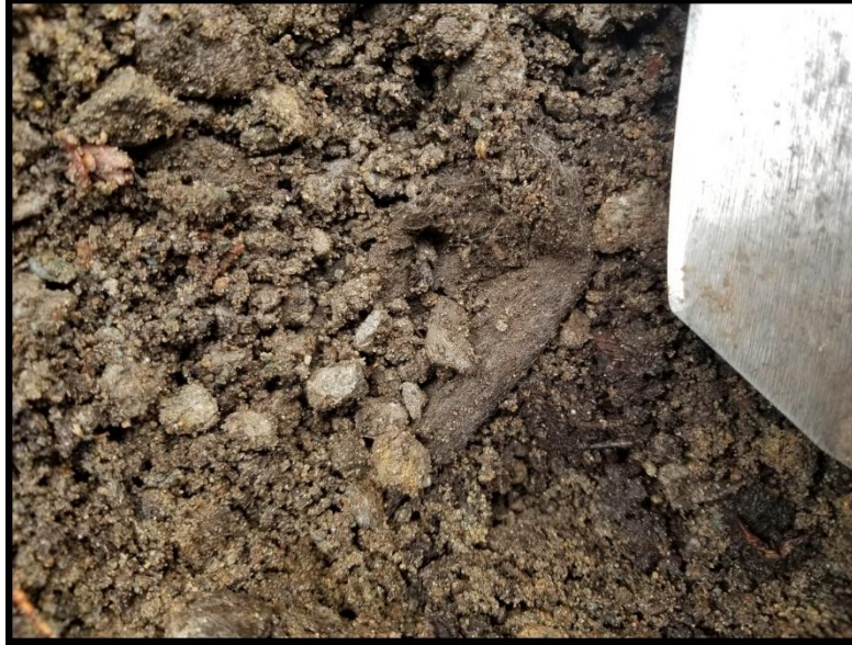
Image 7. Photograph 3418 of a test pit dug in the centre of the study area, showing geotextile under allogenetic granular material, and over bedrock.
