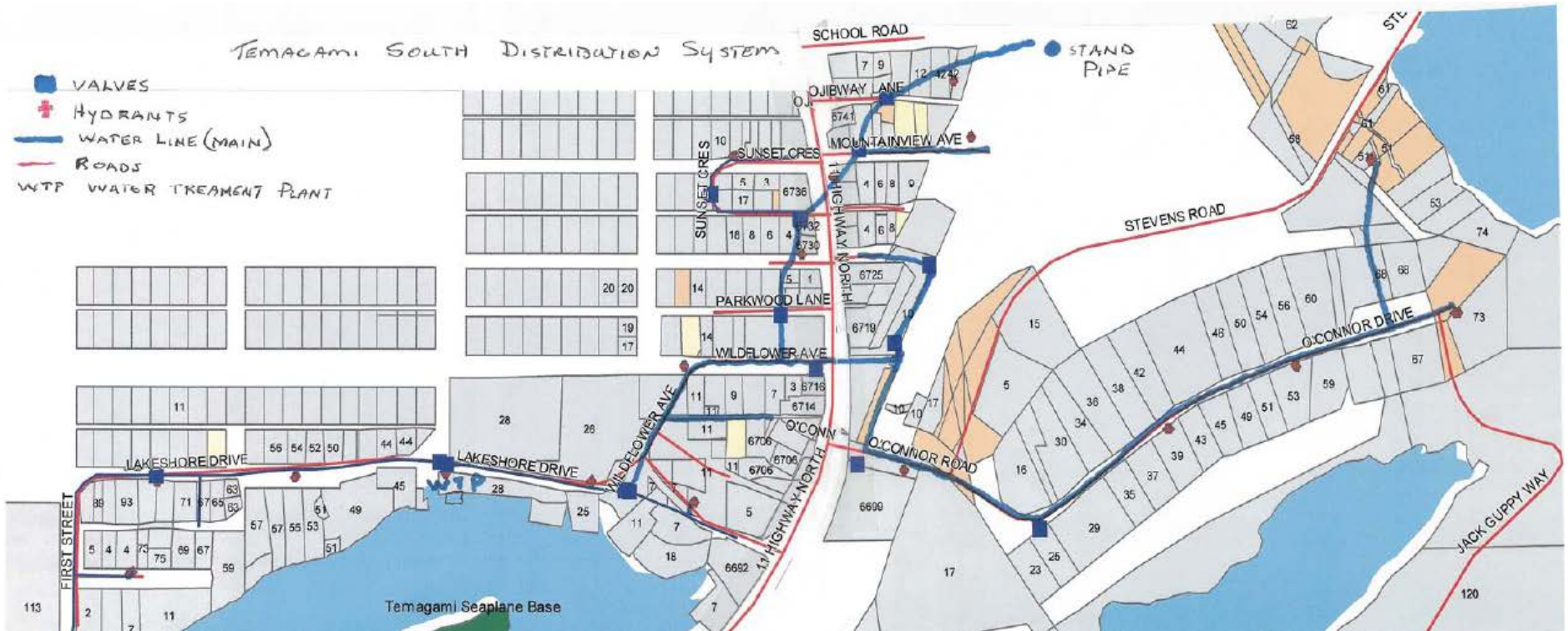
Figure 2 - Temagami South Distribution System Map. Larger scale version available at the Temagami Public Works office
