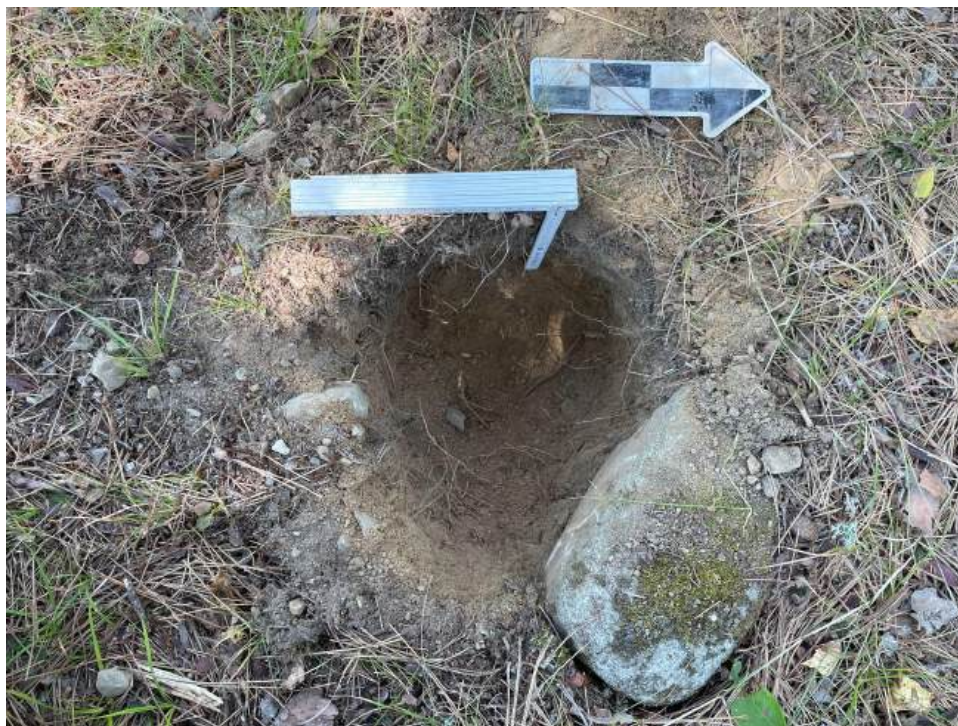
Image 5: Representative test pit showing sandy soils.
