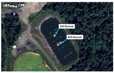
The Biofixe modules are operating well, providing good overall quality effluent with respect to the removal of BOD, TAN, TP and TSS. Once more data is available with all four blowers in operation, an assessment can be made to determine the system's optimal effectiveness.
